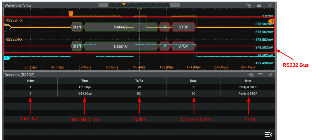
Figure 21.6 RS232 Decoding Event Table
