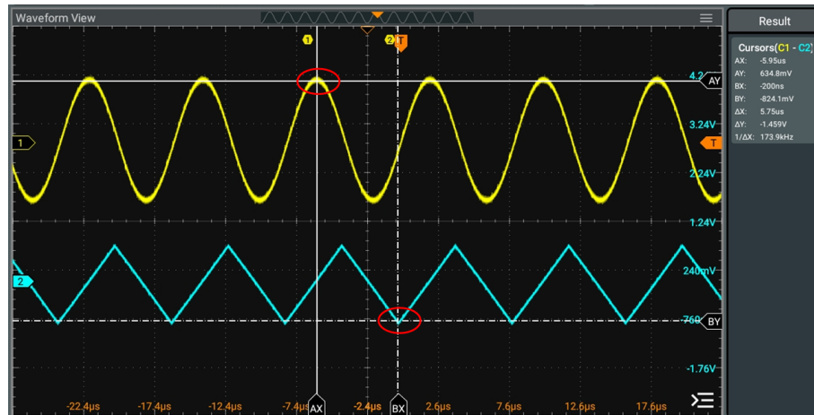
Figure 10.10 Track Measurement (before Horizontal Expansion)
